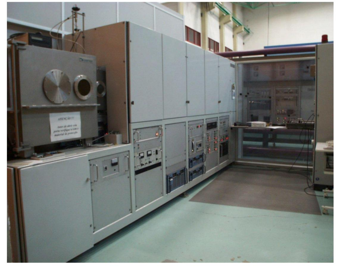
IST-ID 210 kV ion implanter has a chamber allowing the implantation of an area of  $20 \times 20 \text{ cm}^2$ , and to carry on implantation samples in the temperatures range of 77 K up to 1273 K, in a controlled way.
