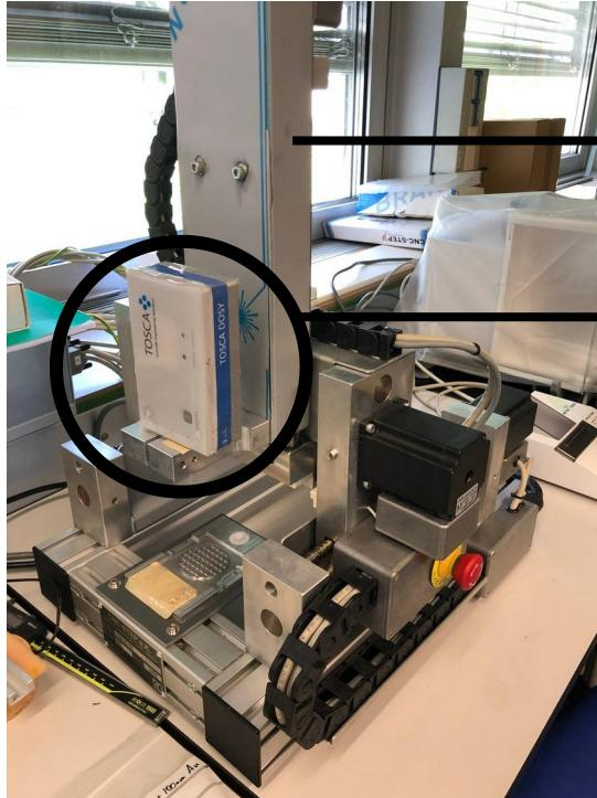
→ 3D positioning system (automatic movement)
