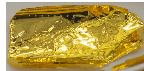
After the lift-off, the Au doposited remains only on the Absorber
