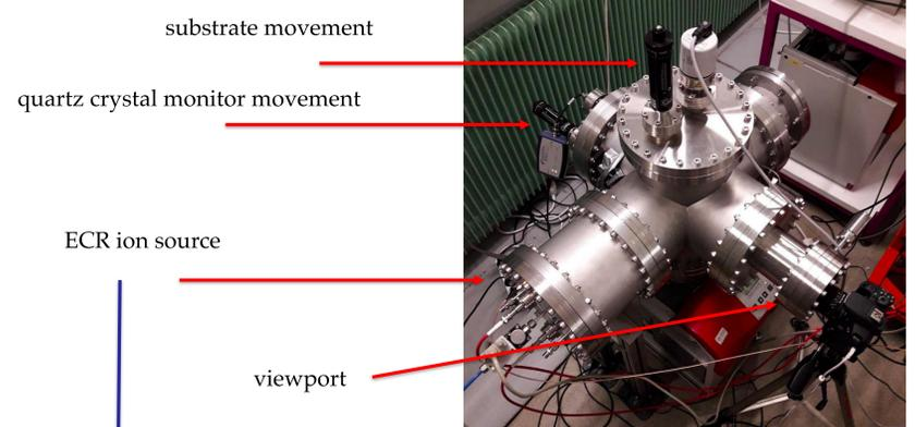
Left: ECR ion source with control electronics
