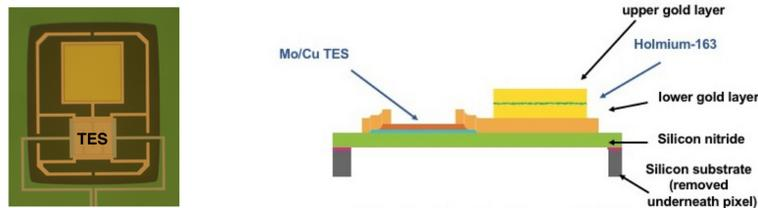
Top : sketch of the current pixel design, including all processing steps. The detectors will be fabricated at NIST up to the bottom half of the gold absorber, then in Italy the absorbers will be completed with Au: $^{163}\text{Ho}$  implantation/final gold deposition to fully encapsulate the isotope and, finally, the silicon nitride membranes will be released by deep etch of the silicon on the backside of the array.
