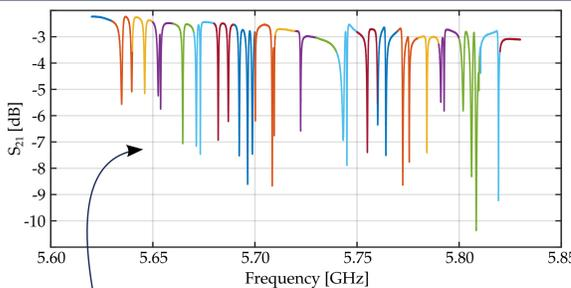
33 available multiplexed channels; μMux chip (multiplexing) IF Board (Rshunt)
