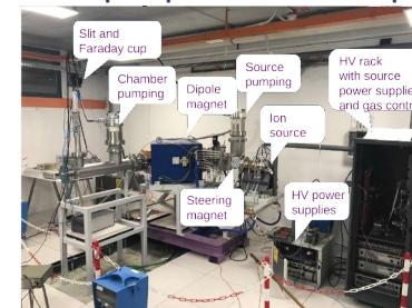
Ion implanter equipped with Ar sputter ion source and magnetic dipole + electrostatic quadrupole (later) for a  $^{163}\text{Ho}$  beam with 4 mm FWHM spot and mass separation  $163/166$  better than  $5\sigma$ .
