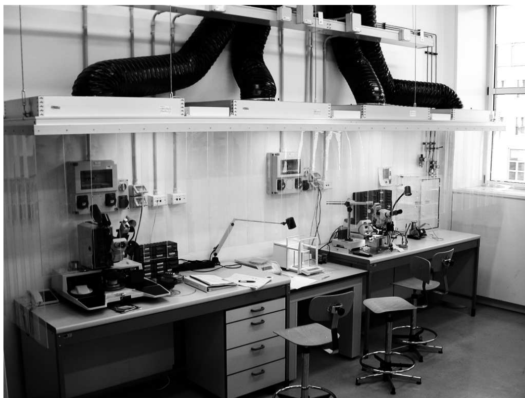
Figure 5.19 - View of the ISO 6 work area in Milano for \text{AgReO}_4 crystal detectors preparation with wire-bonder, precision balance, micropositioner and dry box.
