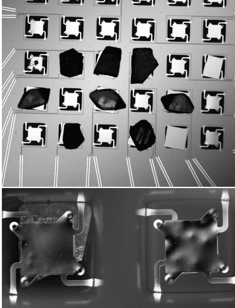
Figure 5.23 - XRS2 array: view of several pixels with \text{AgReO}_4 absorbers (top); single element close bottom view (bottom).
