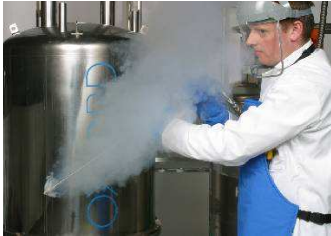
Figure 4 Operator is protected from cold helium gas by gloves and face mask
