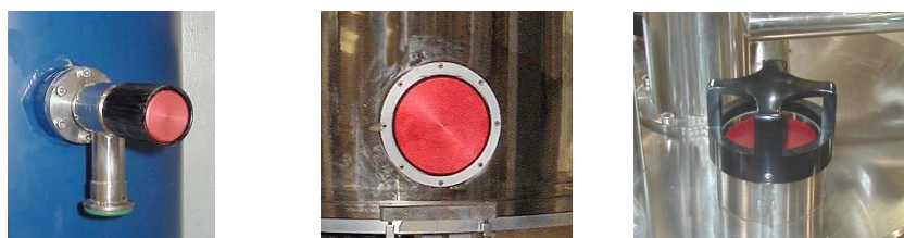
Figure 1 Examples of Oxford Instruments (red) over-pressure relief mechanisms
