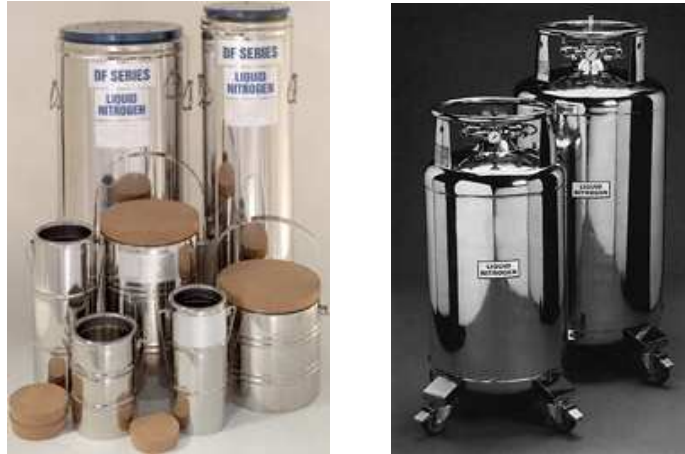
Figure 5 Examples of open and self-pressurising liquid nitrogen storage vessels 2 .
