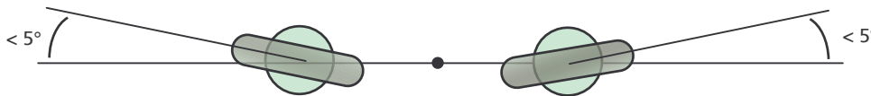
Figure 17 The plane of the eyes of a pair of collar eyebolts should be within \pm 5^\circ of the plane containing the centre of gravity and the axes of the eyebolts
