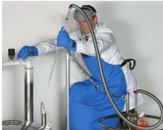
Figure 3 A full set of PPE including cryogenic apron and gloves and face mask 2
