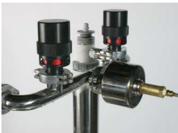
Figure 11 A pair of pressure relief valves fitted to an Oxford Instruments NMR system
