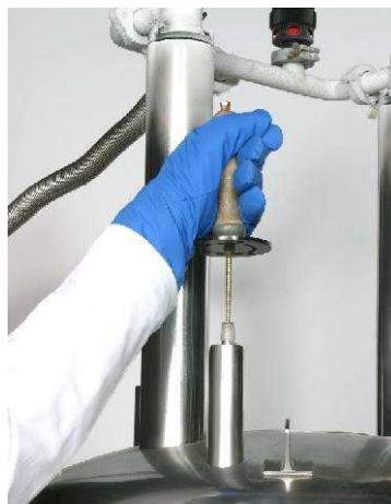
Figure 13 Check for nitrogen vessel blockages regularly and often and clear them as soon as possible
