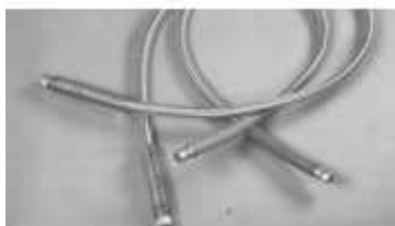
Figure 7 Stainless steel transfer lines for liquid nitrogen 2 .
