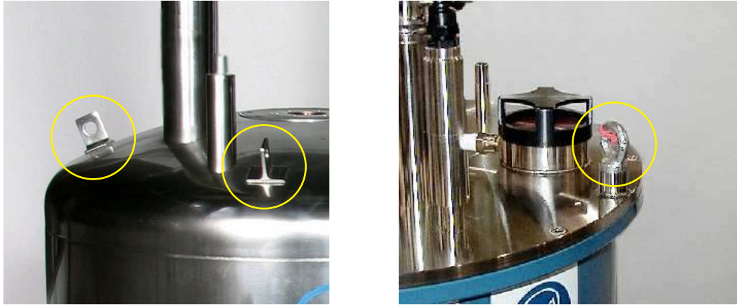
Figure 16 Lifting lugs and eyebolts as fitted to Oxford Instruments systems
